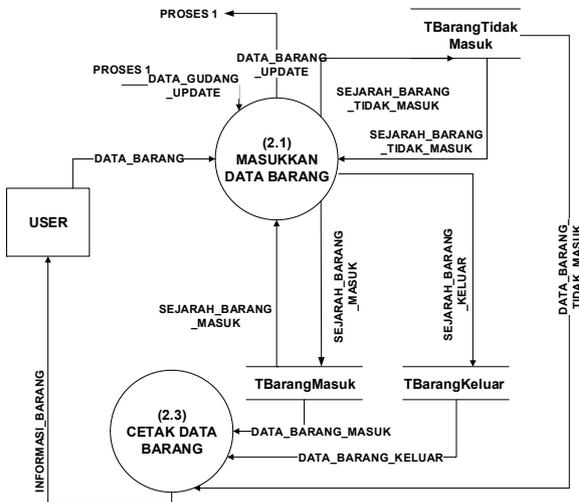
Gambar 8. Data Flow Diagram Level 2 Proses 2
